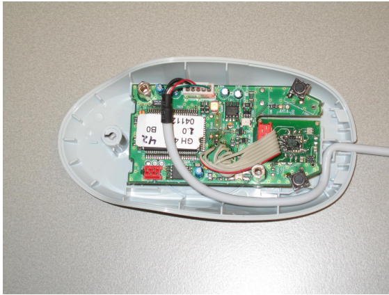
Fig. 15. Retrofitted mouse with TELEMUS sensor
