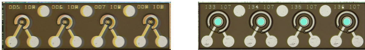
Figure 2. Top view of an flip-chip 1x4 top-emitting VCSEL (left) and top-receiving photodiode (right) array die.
